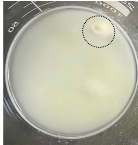
CK Brand: Slow disintegration, Formation of gelatinous mass during dissolution (dotted circle)
