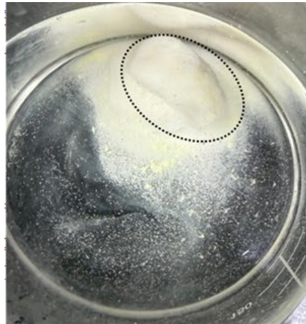
CK Brand: Slow disintegration, Formation of gelatinous mass during dissolution (dotted circle)
